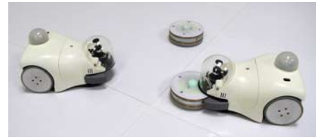
Figure 9. The Cyber rodent: robotic platform for assessing how the reward system should be designed and how it can be evolved (Doya and Uchibe, 2005). The marked features of Cyber Rodents are the capabilities to capture battery packs for survival and to exchange programs by infrared transmission for software reproduction.
