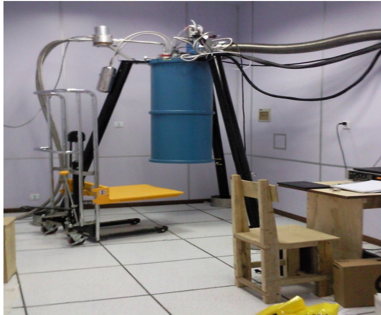
Cryofree dilution refrigerator: <15\text{mK}
