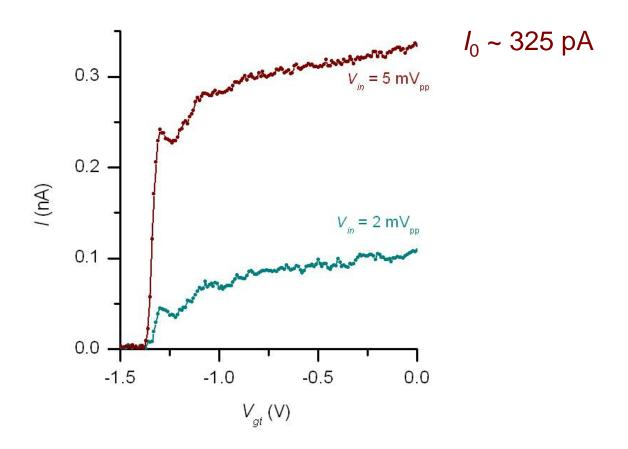
For 5 mV<sub>pp</sub>,  $I_0$  is similar to that at 1.2 K, 2 mV<sub>pp</sub>... but the peak is still visible:
