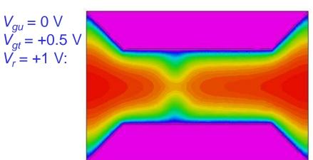
At negative gate voltage we may form a potential barrier between reservoirs:
