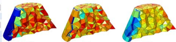
Different mesh quality measures lets you assess the quality of the mesh before solving. Better quality measures can often give faster convergence. Different mesh quality measures are suitable for different types of physics
