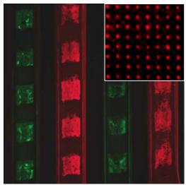
Devices are fabricated as an array of ink having superior life-time to biomolecules. Biomolecules are grafted at the time of use. Main figure shows a prototype multiplex device integrated with microfluidic delivery, green and red represent two different proteins. Inset shows array of 200 nm dots of antibodies.
