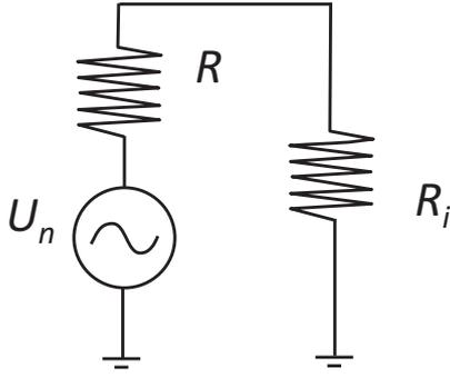
FIG. 3: Thermal noise source loaded onto the input impedance of amplifier  $R_i$ .
