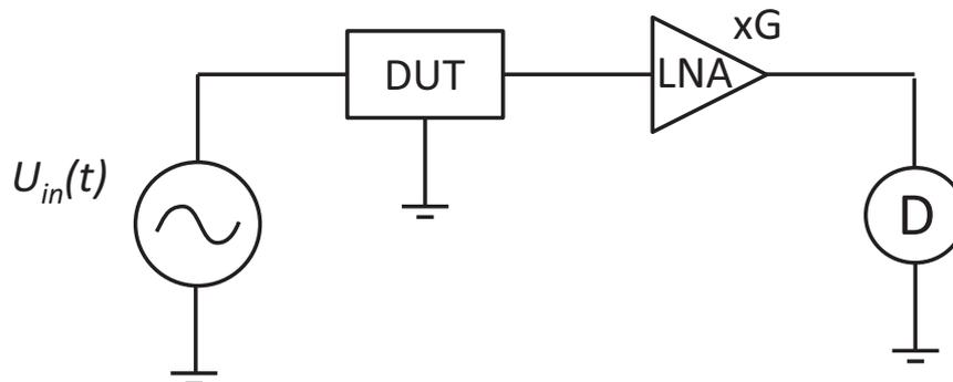
FIG. 1: Typical RF measurement setup which includes a low-noise amplifier (LNA).
