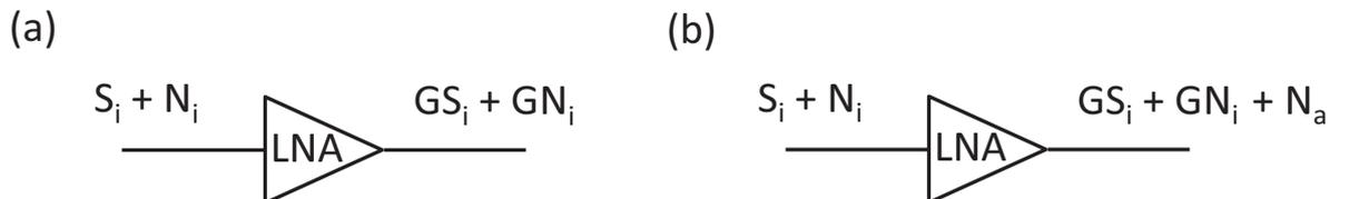
FIG. 2: Input and output of an ideal (a) and real (b) amplifier.
