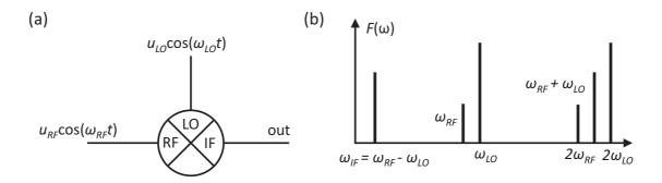
FIG. 1: Down-conversion mixer (a) and the power spectrum of its output (b).
