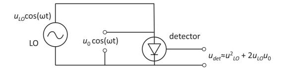
FIG. 3: Schematic of the homodyne detection.
