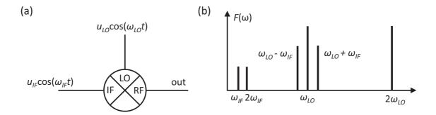
FIG. 2: Up-conversion mixer (a) and the power spectrum of its output (b).
