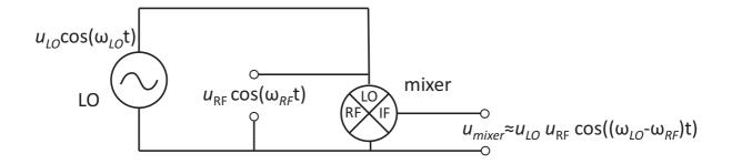
FIG. 4: Schematic of the heterodyne detection.
