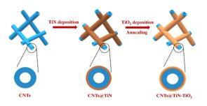
Controlled deposition of TiN and  $TiO_2$  layers on CNT sponge by ALD. The resulting Li-S battery has enhanced cycling stability and aerial capacity.
