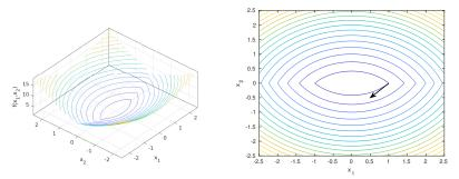
3D plot (left) and level sets (right) of  $f(\mathbf{x}) = \max[x_1^2 + (x_2 + 1)^2, x_1^2 + (x_2 - 1)^2]$ . A negative subgradient is indicated by the black arrow
