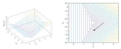
3D plot (left) and level sets (right) of  $f(\mathbf{x}) = \max[-x_1, x_1 - x_2, x_1 + x_2]$ . A negative subgradient is indicated by the black arrow
