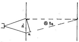
The difference a between the trajectories 1 and 2 of the electron, causes the phase difference
