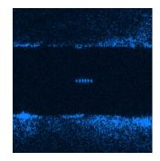
Figure 2. 6 laser cooled single Calcium ions between the electrodes of the ion trap above
