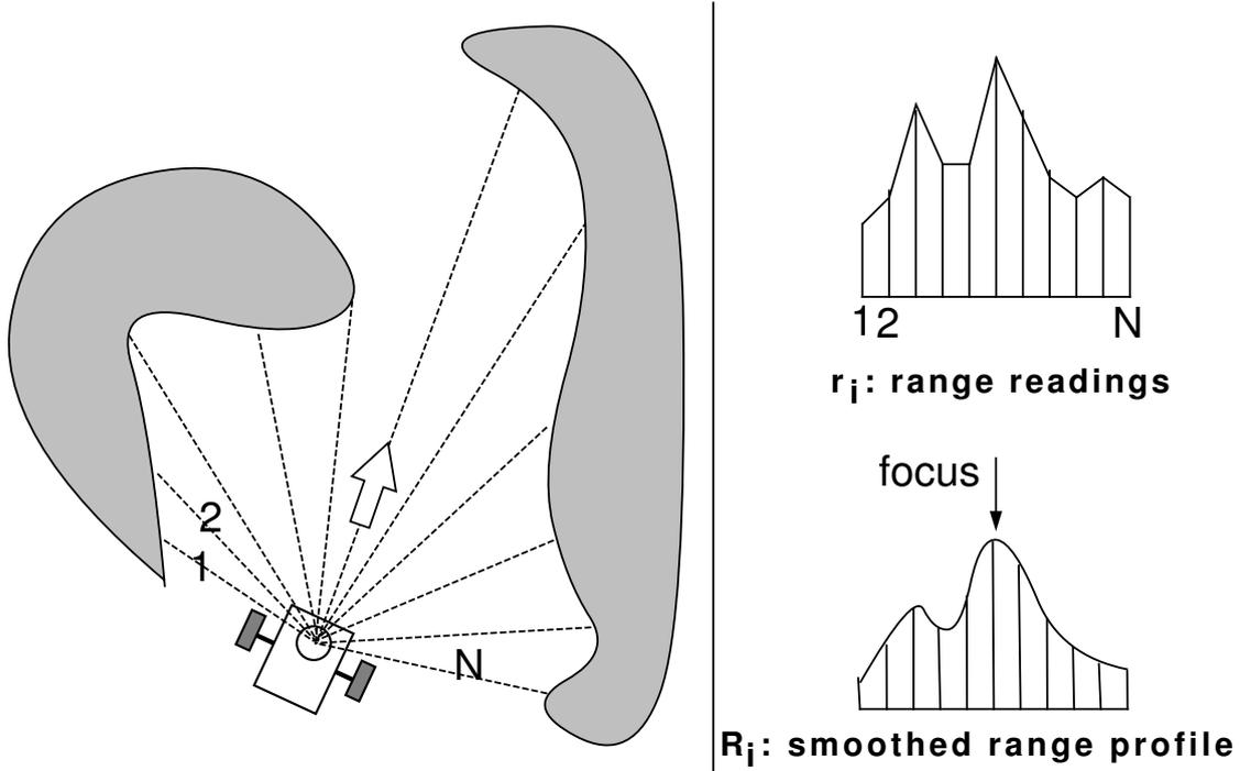
Figure 2: The Range profile is obtained from the frontal side of the robot. The robot moves by tracking the maximum in the range profile.
