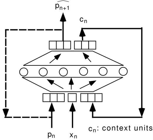
Figure 5: Forward model using the RNN architecture. The dotted line indicates the closed sensory loop which is used for lookahead prediction in multiple steps.
