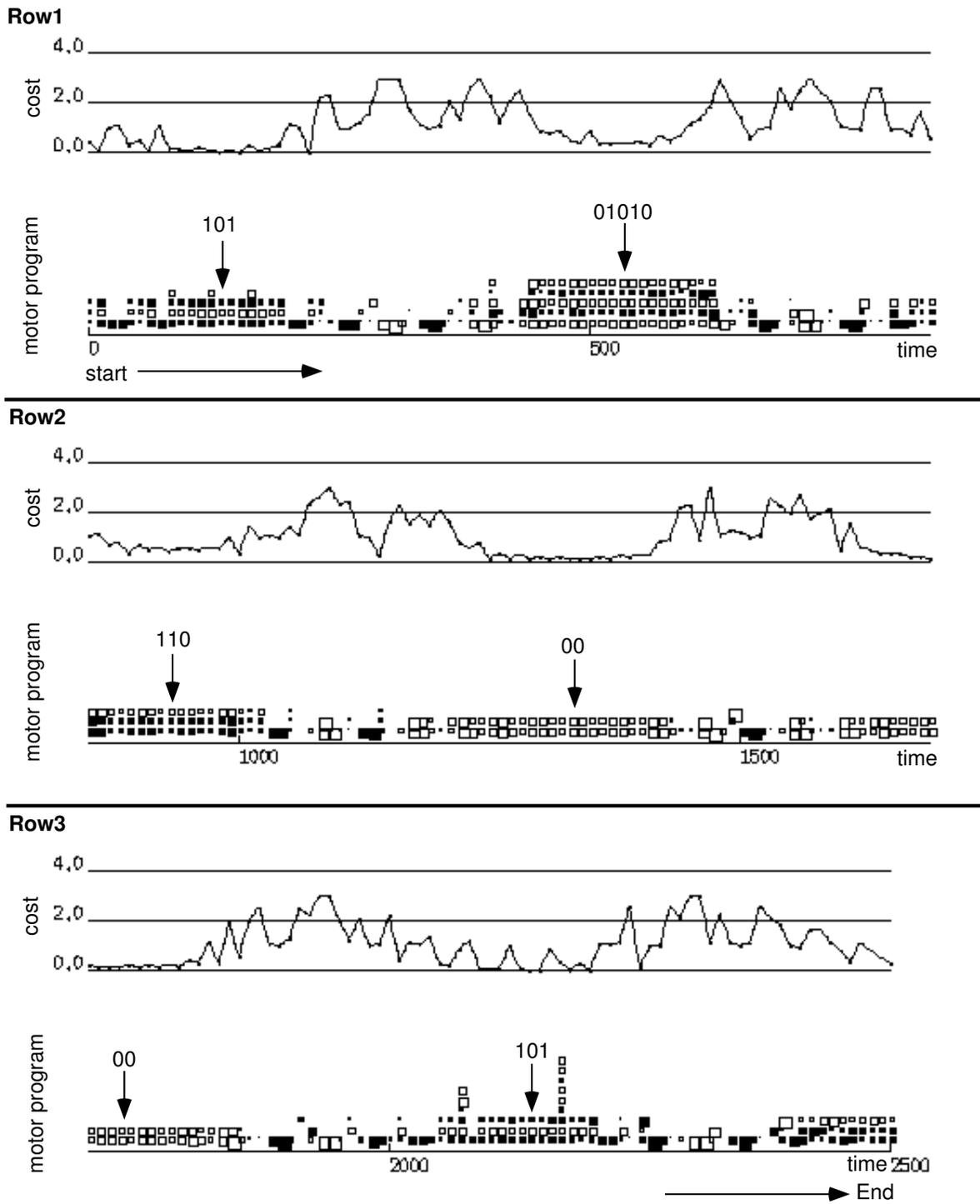
Figure 10: The chaotic search process of the motor program is shown in the three rows. In each row, the upper part indicates the cost time history, and the lower part the temporal motor program. The temporal motor program is indicated by a column consisting of black and white squares, representing motor commands of 1 and 0 respectively. The motor programs obtained in the stable phase (101, 01010, 110, 00) are indicated by arrows. Time flows from row 1 to row 3.
