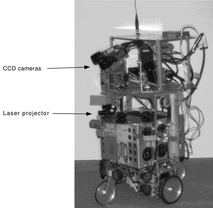
Figure 1: The *YAMABICO* mobile robot equipped with a laser range sensor.
