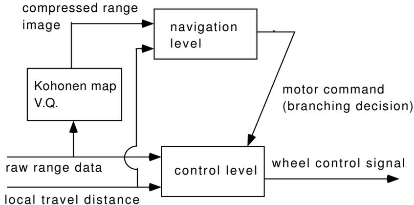
Figure 4: The navigation architecture employed here, comprising the control and navigation levels.
