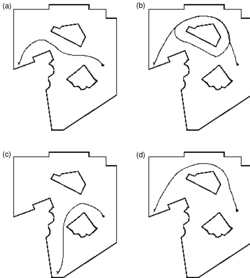
Figure 11: Travels based on various motor programs. (a) and (d) are almost optimal trajectories, (b) is redundant, and (c) pursues the wrong goal. (a), (b), (c) and (d) correspond to the motor programs 101, 01010, 110 and 00, respectively.
