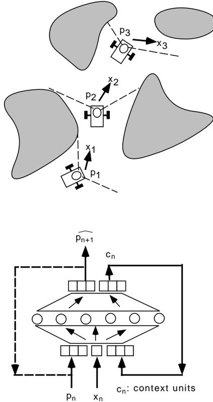
Figure 2: Sensory-motor sequence in branching and RNN architecture.
