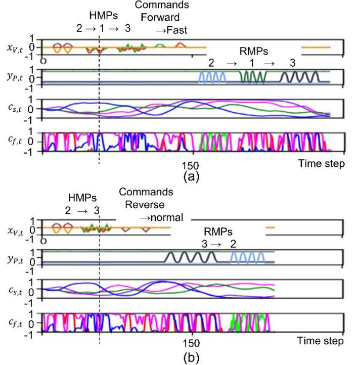
Fig. 4. Two examples of test trial results in (a) and (b), plotted with the slow context units activity.  $x_{V,t}$ ,  $y_{P,t}$ ,  $c_{s,t}$  and  $c_{f,t}$  indicate the vision (Kinect) inputs, the motor (proprioception) output, and the slow and fast context units activities.
