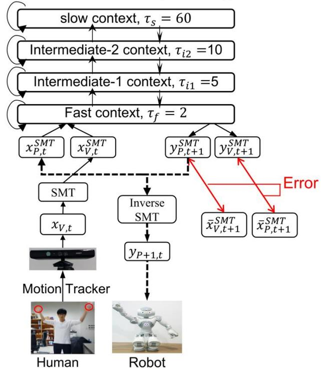
Fig. 1. The whole system architecture for the performing the communicative tasks with MTRNN. SMT denotes softmax transformation.  $x_{V,t}^{SMT}$  and  $x_{P,t}^{SMT}$  are the vision and proprioception inputs at time step  $t$ , respectively.  $x_{V,t+1}^{SMT}$  and  $x_{P,t+1}^{SMT}$  are vision and proprioception prediction outputs,  $y_{V,t+1}^{SMT}$  and  $y_{P,t+1}^{SMT}$  are their targets.  $\tau$  is the time constant of the context unit.
