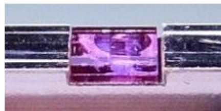
Schematic of a nitrogen doped diamond implemented as a maser amplifier
