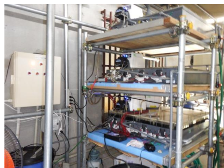
Prototype MFC at distillery operating continuously since 2013
