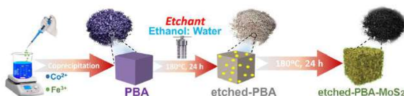
Figure 1: Schematic representation of designing etched-PBA-MoS 2 for CO 2 reduction reaction.
