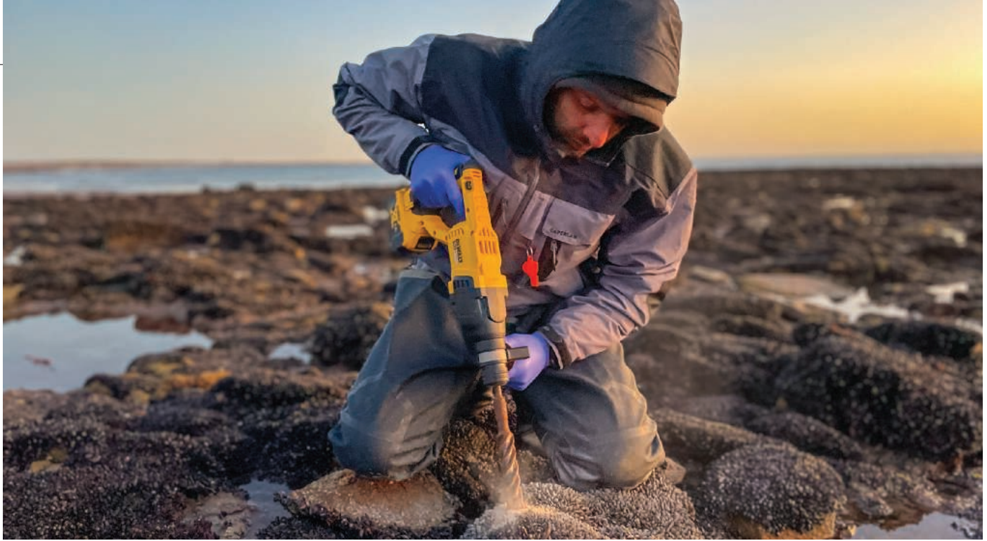
Researcher Rui Seabra drills a hole for securely mounting a sensor near Puerto Lobos, Argentina. The devices can record hourly temperatures and store data for up to 15 years, enabling scientists to assemble a detailed picture of the intertidal zone's thermal characteristics.
