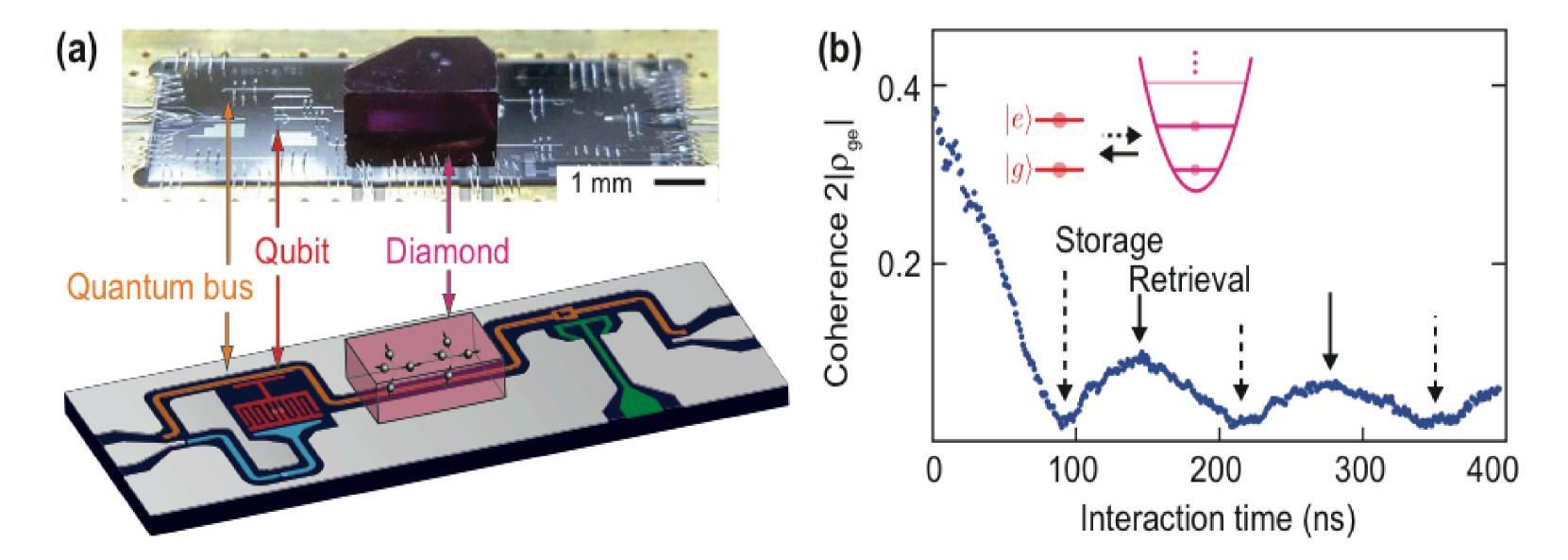
(a) Photo (top) and schematic (bottom) of the hybrid quantum circuit. A transmon qubit (red) is coupled to an ensemble of NV centres electron spins (pink) via a frequency tunable quantum bus resonator (orange). (b) Modulus of the off-diagonal element  $r_{ge}$  of the qubit density matrix as a function of interaction time with the spin ensemble.
