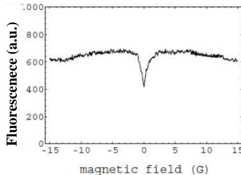
Coherent population trapping on the  $D_1$  line of a thermal sodium beam
