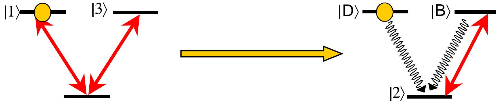
Coherent population trapping in two-electron three-level systems with aligned spins
