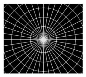
Fig. 3. The static field with the propagating spherical wavefront and field lines. Snap shot from the Radiation 2D simulator.
