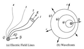
Fig. 1. Electric field lines of moving charge, and spherical wave-fronts.
